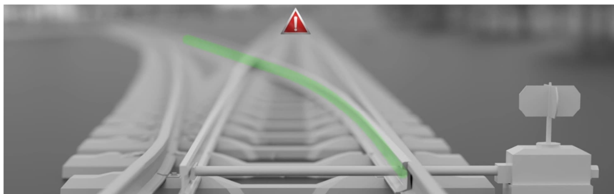
Figure 3 Broken rail alerting control center to use rail interlock to divert following trains for damage prevention.
